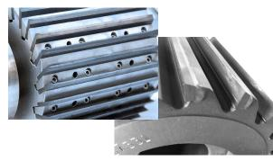
AMERICAN CUTTING EDGE offers a three-step resurfacing and sharpening process specifically for pelletizer rotors that helps preserve proper geometry to improve overall blade life and cutting efficiency – protecting your bottom line. For best results we suggest that you send in your rotor for review. Upon review, we'll recommend a grinding profile that will improve the overall life of your pelletizer rotor.
